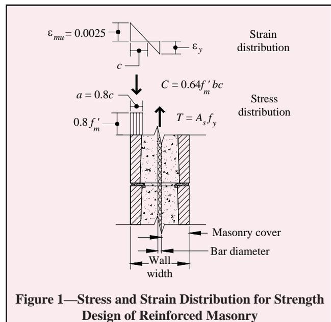
**Figure 1—Stress and Strain Distribution for Strength Design of Reinforced Masonry**
